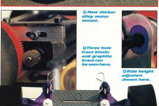
O Alloy diff spacer can be seen behind the plastic nut. This replaces the old thrust race and makes the differential a lot smoother.
